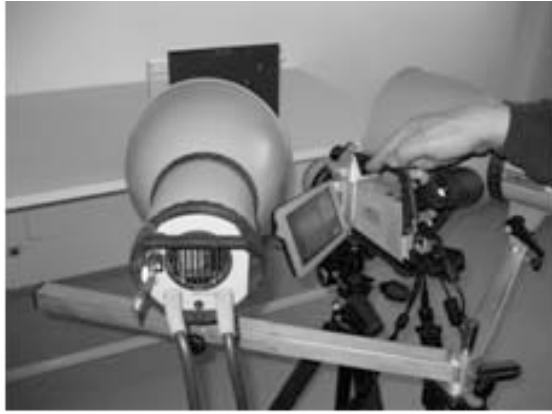
Figure 7. Test arrangement for the pulsed thermographic (flash method) measurements.
